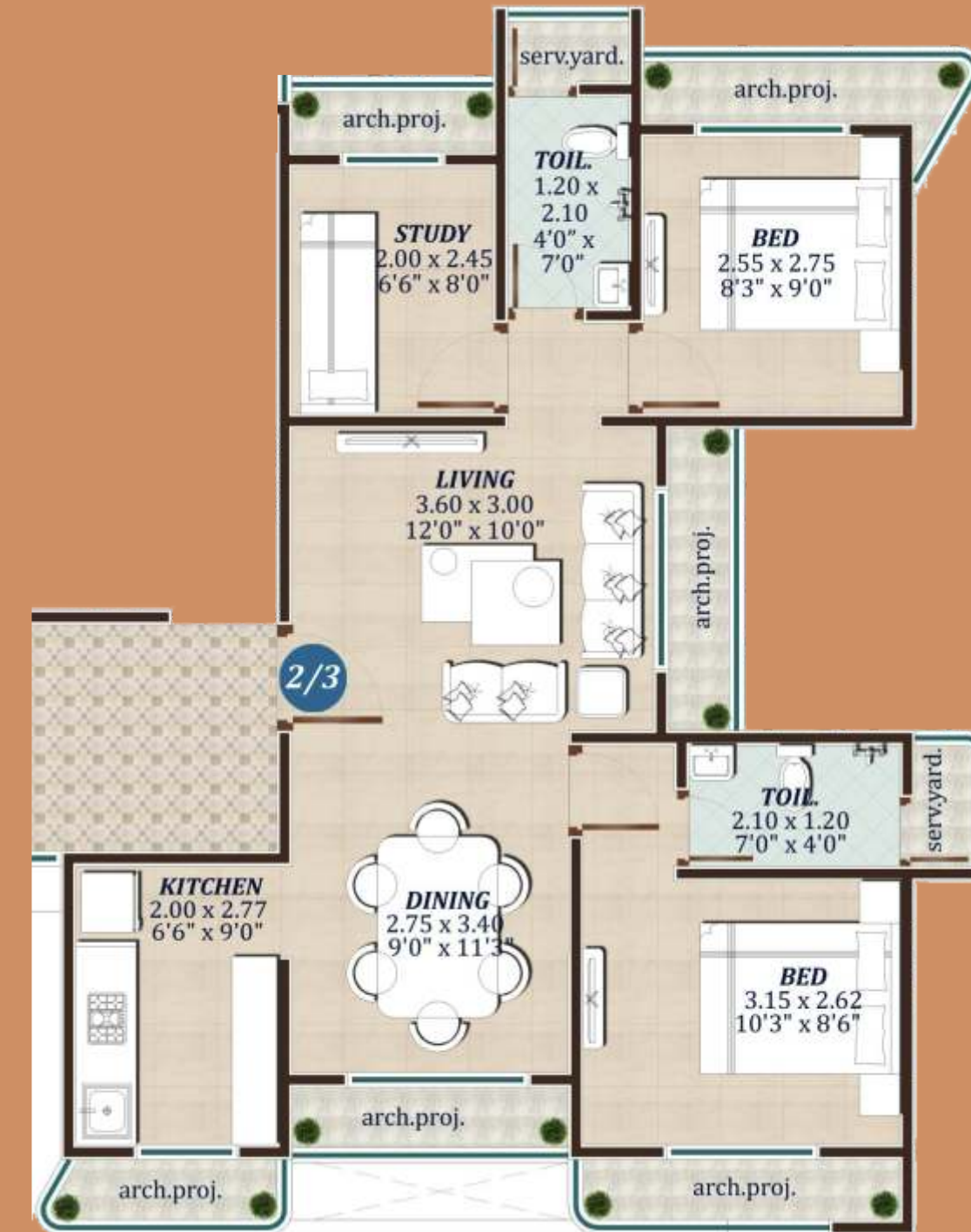
JOINT FLAT No. 2 & 3 ISOLATED VIEW
