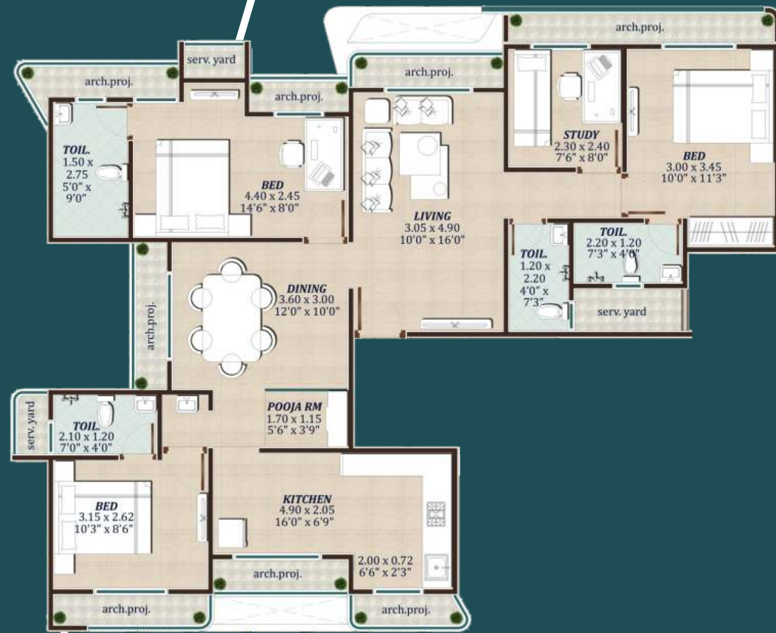
JOINT FLAT No. 6, 7 & 8 ISOLATED VIEW
